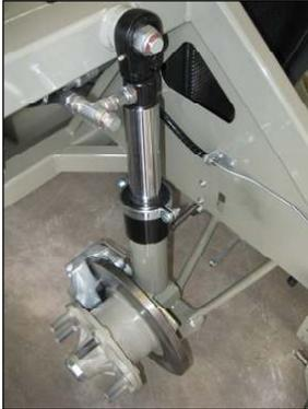
The four independent suspensions, whose regulation and control is assigned to an electronic control unit, are hydraulic with McPherson system on all four-wheels. Each wheel has a hydraulic cylinder and accumulator which ensure optimal absorption of road surface irregularities without using springs.
