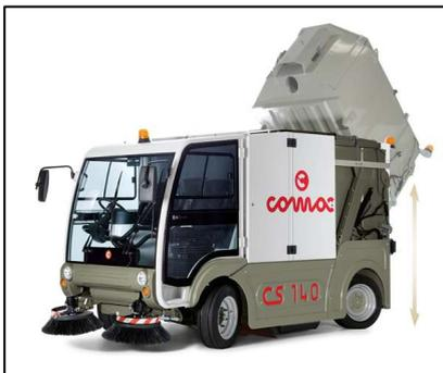
The total volume is approximately 3,5 m<sup>3</sup>, a capacity which reduces the down time required for emptying and therefore also the total cleaning time. It is vertically divided in two parts the lower part is designed for collection of material while the upper part houses the filter. The waste hopper is emptied by lifting it on vertical guides up to 1.800 mm.
