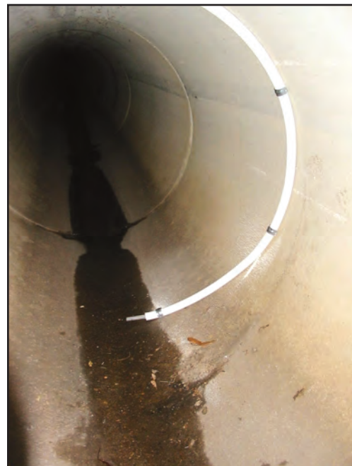
Figure 22. Water-quality sample intake located at a fixed point along the storm-sewer wall.
