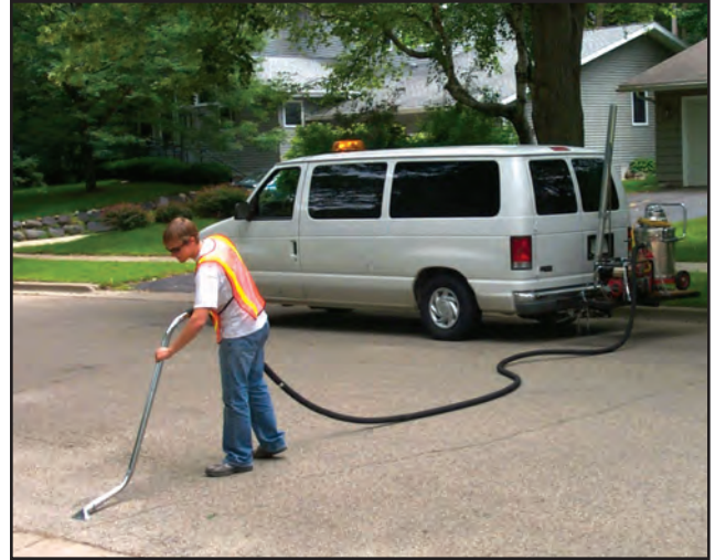
Figure 2. Demonstration of equipment used to collect street dirt samples.
