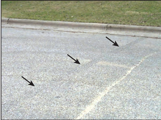
Figure 3. A vacuumed strip leaves a visible trail indicating the degree of available street dirt.
